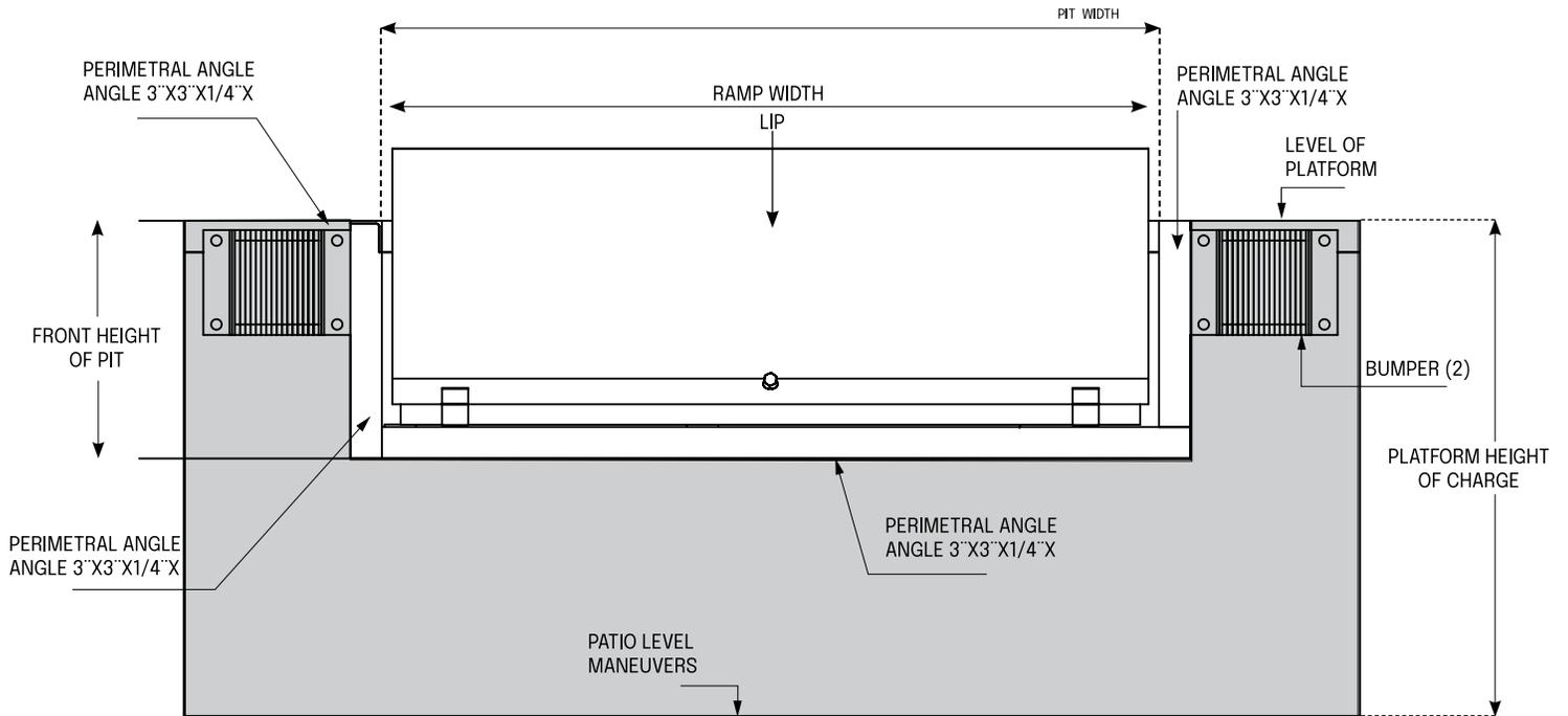
The safety stop included in the lip of the hydraulic levelers consists of an extension of the lip of the hydraulic leveler itself.
