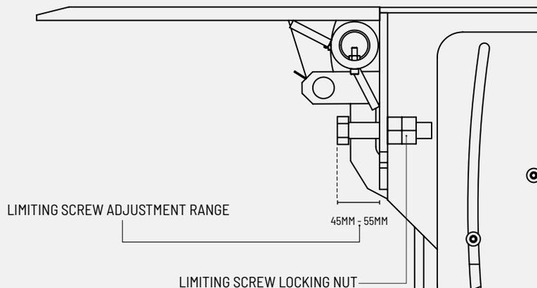
1. loosen the locking nut on the limiting screw.
