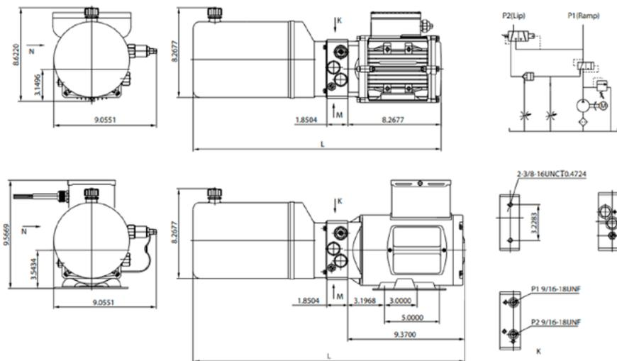
This platform leveler power unit raises the ramp when the motor is activated, when the ramp has reached the maximum extension level, the sequence changes to extend the lip. The ramp and lip are lowered by separate solenoid valves during lowering.
